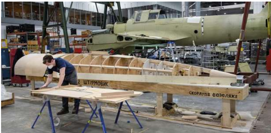
Restoration specialist Jay Flanagan re-builds the wooden rear fuselage utilising a wooden mold.
