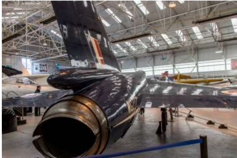
A rear view of WG777 showing the variable area tailpipe.
