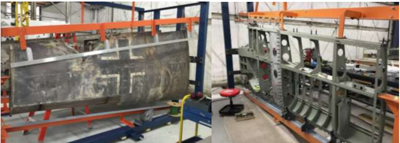
A wing assembly jig in use before and during the restoration process.
